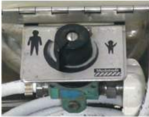
Figure 14: Close up of the modified Robertshaw valve, fitted to the Oxy-Viva.
