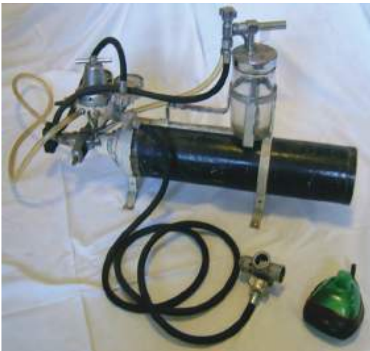
Figure 5: CIG Emergency Oxygen Outfit (TM8), with RM fitted.
