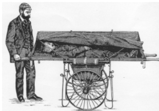
The extraordinary 'Furley-Headley' litter. It could carry two patients sitting (left) or one lying (right), and the legs could be raised and lowered. How stable it was when carrying two patients is a matter that invites speculation.
