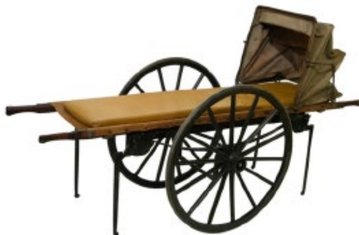
The iconic Ashford Litter. Marketed by the Ambulance Department of the Order of St John from 1879, it continued being sold by the St John Ambulance Association until at least 1939. Over time, various improvements were made, the first being the addition of the fold-up hood fitted to the litter in this photograph.
